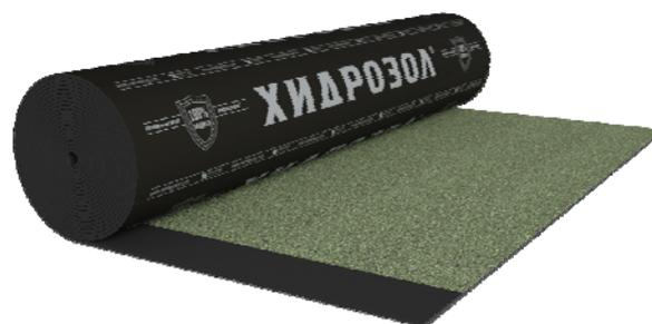
The fiberglass reinforcement significantly improves physical-mechanical properties of the membrane as it increase its strength and resistance to tear and puncture. Even when the membrane is cut or torn off the reinforcement keep the membrane intact and prevent its further damage. The glass veil provides dimensional stability of the bitumen at low and high temperature, as well as it guarantees the maintenance of the initial form even when subjected to extremely high loadings.
